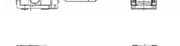
K-V-B-Y 底脚花键空心轴 (DIN5480)安装斜齿轮— 伞齿轮减速电机 K Series Foot-Mounted/Splined Hollow Shaft (DIN5480) Helical Gear Unit
